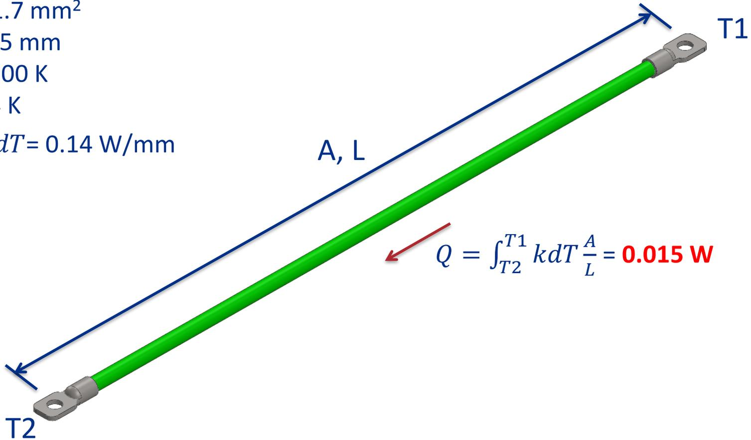
$$Q = \int_{T_2}^{T_1} k dT \frac{A}{L} = \mathbf{0.015 \text{ W}}$$
